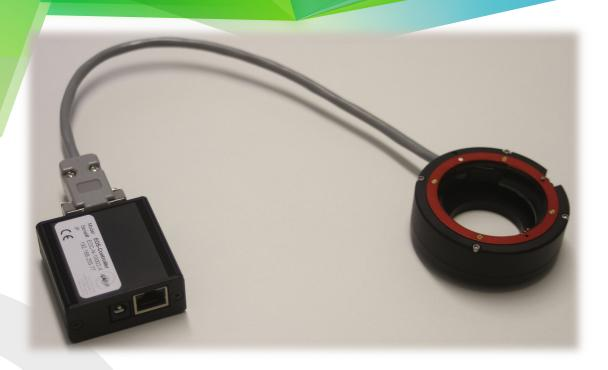
The ILA\_5150 EOS Lens Controller allows remote control of Canon EOS lenses via software over standard ethernet giving the user the freedom to use long cables and the existing network structure. The ILA\_5150 EOS Lens Controller takes command of the motors and encoders built into the lenses, for fast, precise and trouble free focus and aperture control.
